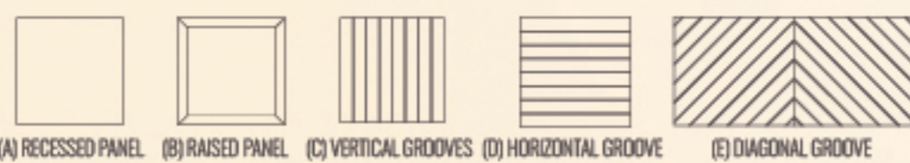
(A) RECESSED PANEL (B) RAISED PANEL (C) VERTICAL GROOVES (D) HORIZONTAL GROOVE (E) DIAGONAL GROOVE
